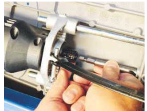
The drills are held in a sleeve chuck for quick changeover
